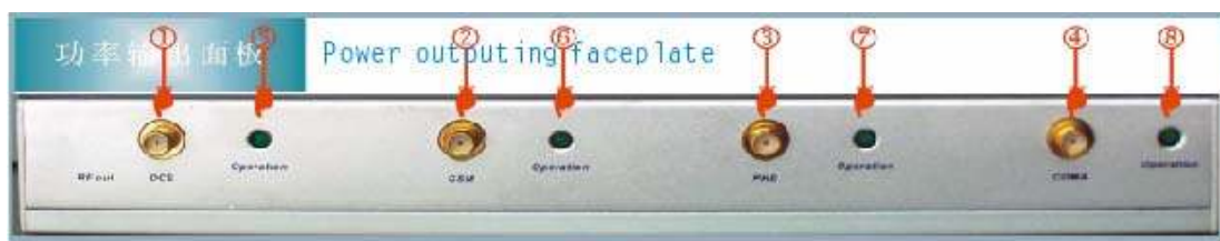
①/②/③/④: DCS/GSM/PHS or 3G/CDMA RF outputting port(connect antenna) ⑤/⑥/⑦/⑧: DCS/GSM/PHS or 3G/CDMA pilot lamp of operation
